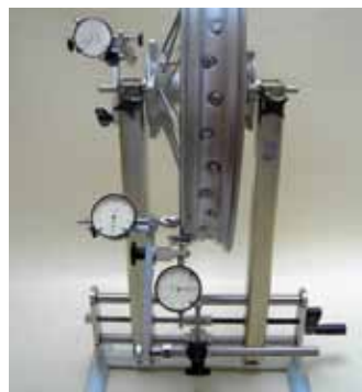
Motorbike model Screwable axle clamp · Span width 300 mm · with adapter for wheel support · Brake disc gauge as an accessory · also suitable for bicycles
